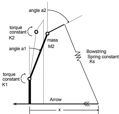
Fig. 5. The Simple bow model (upper limb only).
