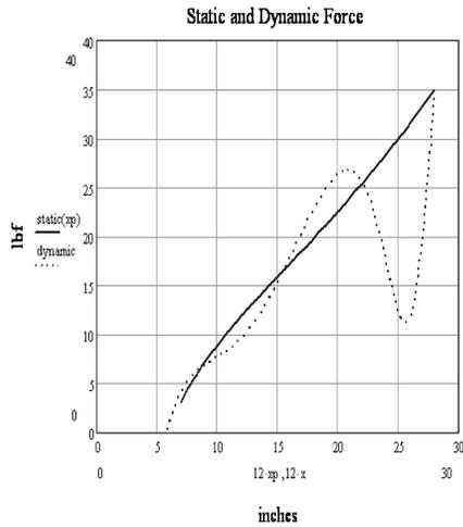
Fig.9. Static and dynamic force on the arrow.
