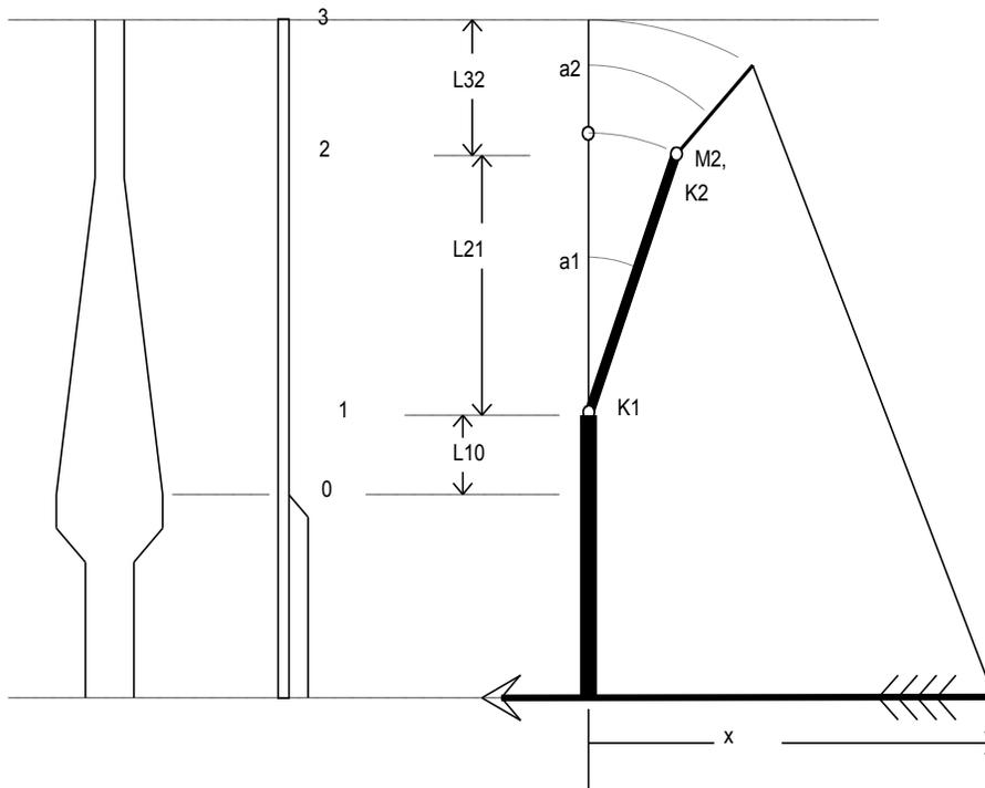
Fig. 7. Modeling parameters for the KL bow.
